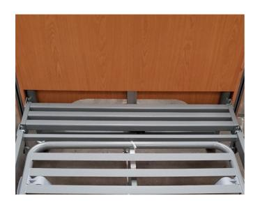
4. Attach the lift system to the sleeping platform/ extension and re-engage the locking pins on the lift system.
