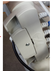
Cable cover unclips/clips into place
