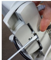
Cable cover unclips/clips into place
