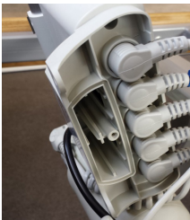
Unscrew/screw the battery cover into place by using the screw provided
